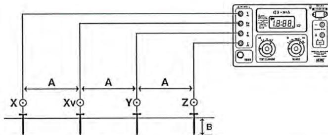
Electrode Spacing (A) 10 ft      Electrode depth (B) 0.5 ft
